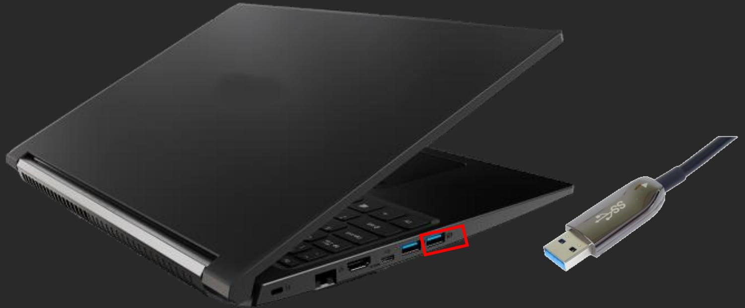
**NOTE:** For the camera to work at maximum performance, plug the camera into the USB 3.0 Port.
